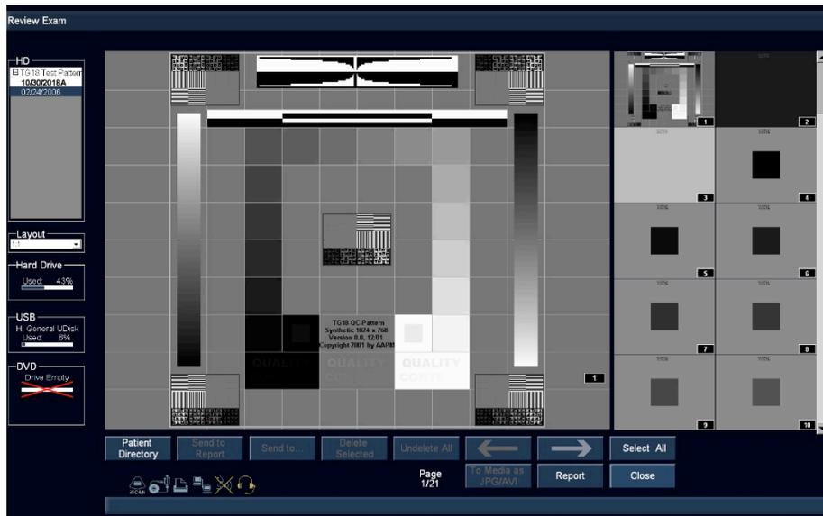
**Figure** SMPTE pattern on the Philips iU22. The Epic 7 will be similar. If possible, enlarge the pattern to fill the entire display.
