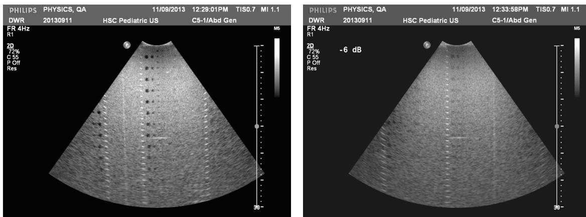
**Figure 2.** Ultrasound image of (left) anechoic cylinders and (right) -6 dB cylinders.
