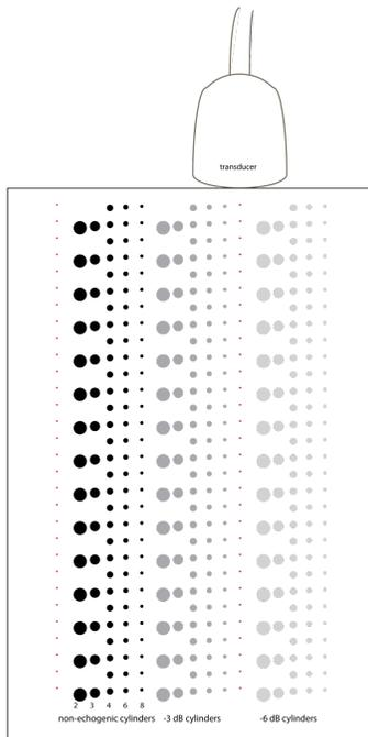
**Figure 3.** For verifying the accuracy of distance measurements in the axial direction, scan the phantom from the top.
