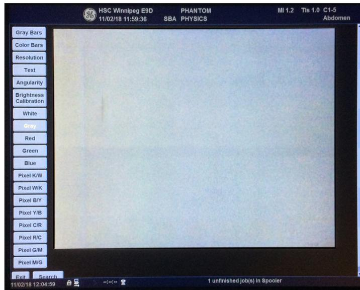
**Figure** Photograph showing the grey uniformity image on a GE Logic E9. Use this to check for bad pixels and other artefacts. In this example a number of streaks are visible and this display may need to be replaced.
