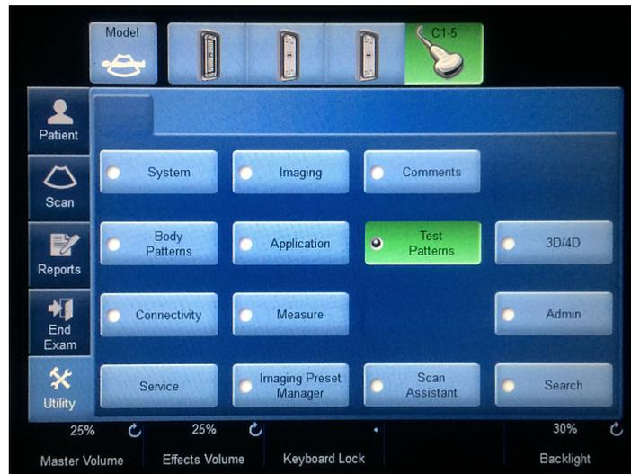
**Figure** Utility menu on GE Logic E9. This provides access to the test patterns.
