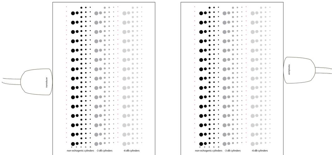
**Figure 4.** For verifying the accuracy of distance measurements in the lateral direction, scan the phantom from either side.
